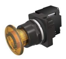
30mm BlackMax, Epoxy Coated Corrosion Resistant Complete Metal Unit Illuminated Push-Pull Operator Transformer type, 240V AC Incandescent Lamp Mushroom Head Cap Small 1 3/4" (44.5 mm) Plastic, Amber 2 Position Maintained, Pull-to-Release UL Listed, CSA Certified NEMA 1,3,3R,4,4X,12,13 & Automotive Standards
