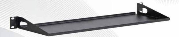
The Kendall Howard Light Duty Rack Shelves are constructed of top gradeu US steel. The Light Duty Rack Shelves come in both solid and vented to maintain proper circulation in your racks and cabinets. Rated to hold up to 45 lbs., this rack shelf is perfect for supporting monitors, switches and other lightweight network or A/V equipment.
