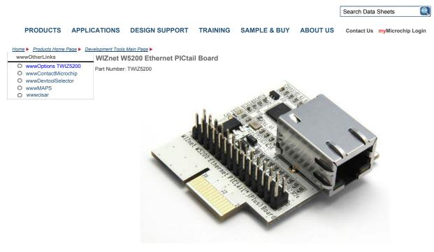
WIZnet's W5200 Ethernet PICtail<sup>™</sup> (Plus) board provides 10/100Mbps, half/full duplex Ethernet connectivity by onboard WIZnet W5200 Ethernet controller, which has a hardwired TCP/IP processing engine.
