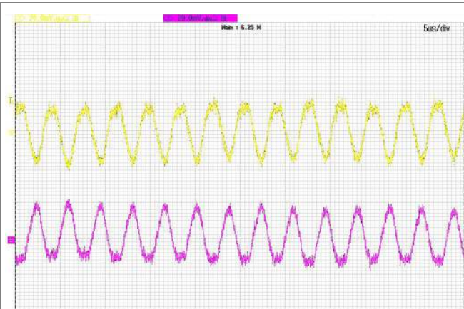
Output voltage ripple at: T_{P1} = +25^\circ\text{C} , V_i = 24 V, I_o = +1.25 A resistive load. Trace: output voltage (20 mV/div.). Time scale: (5 \mu\text{s} /div.). 20 MHz bandwidth
