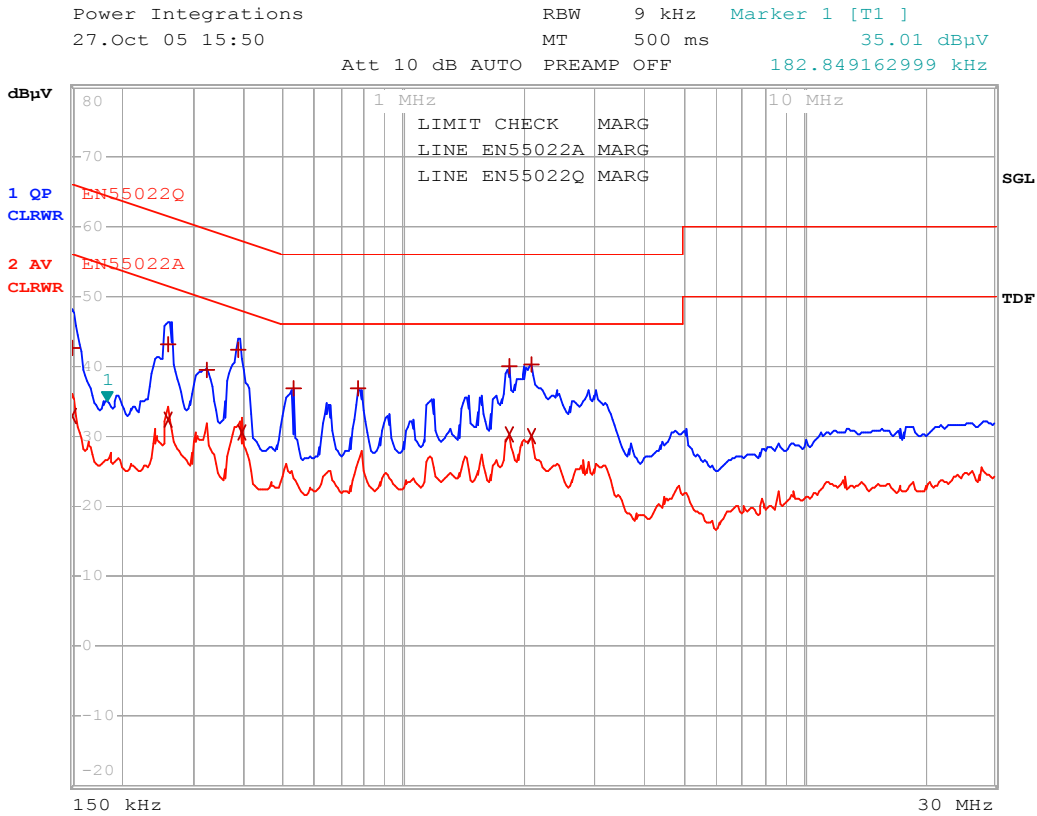
Figure 27 – Conducted EMI, Maximum Steady State Load, 115 VAC, 60 Hz, Artificial Hand and EN55022 B Limits.
