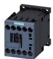
power contactor, AC-3e/AC-3, 9 A, 4 kW / 400 V, 3-pole, 24 V AC, 50/60 Hz, auxiliary contacts: 1 NO, screw terminal, size: S00, upright mounting position
