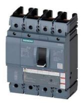
circuit breaker 3VA5 UL frame 250 breaking capacity class H 65kA @ 480V 4-pole, line protection TM230, FTAM, In=150A overload protection Ir=150A fixed short-circuit protection Ii=5...10 x In N conductor protection 100% without connection
