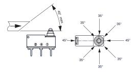
In order to reduce friction and wear, the actuating ramp shall preferably be of PA, POM, PBT or steel, and also be as smooth as possible.
