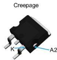
Figure 16. Creepage without top coating
