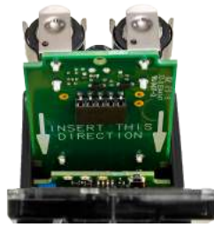
Q45 battery board
