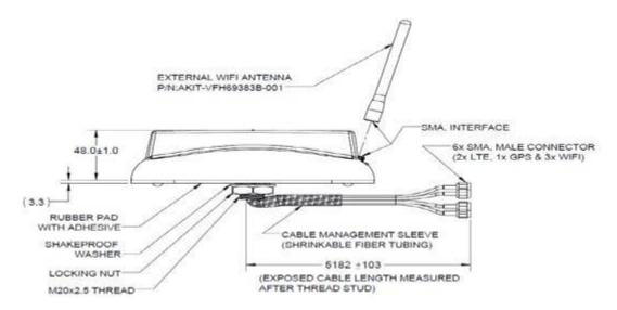
The Barracuda antenna can create an IP67 water-tight seal when installed on vehicles. Certain vehicles such as a Ford Explorer Interceptor have more narrow roof ridges that are tightly spaced together. For this type, vehicle special adapters are available.
