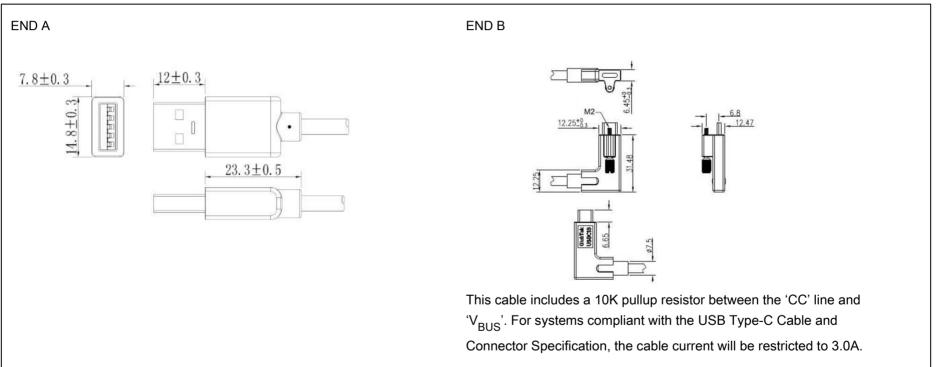
WARNING: The power supply's current rating MUST be  $\geq$ 3.0A to prevent permanent equipment damage and overheating which may result in fire.
