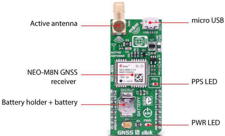
A USB interface (micro USB port), which is compatible with the USB version 2.0 FS (Full Speed, 12 Mbit/s), can be used for communication as an alternative to the UART.
