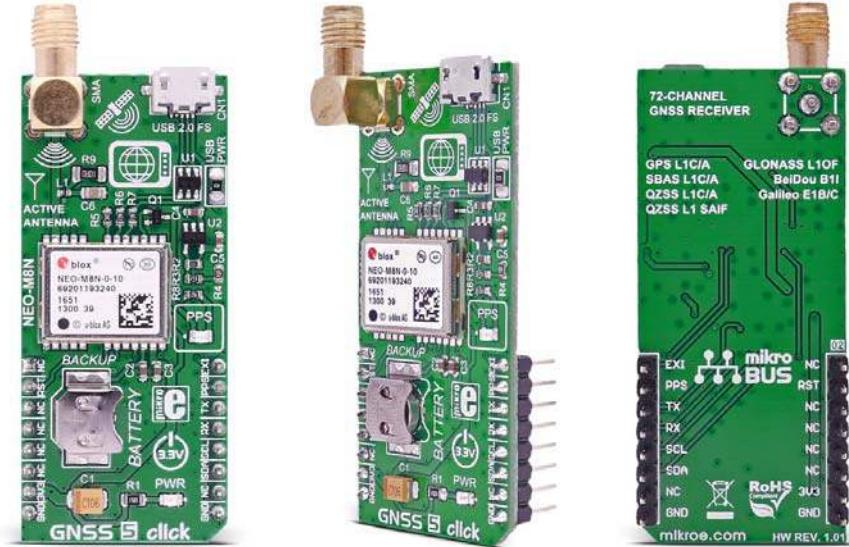
Determine your current position with **GNSS 5 click**. It carries the NEO-M8N GNSS receiver module from **u-blox**. GNSS 5 click is designed to run on a 3.3V power supply. The click communicates with the target microcontroller over I2C or UART interface, with additional functionality provided by the following pins on the mikroBUS™ line: RST, INT, PWM.
