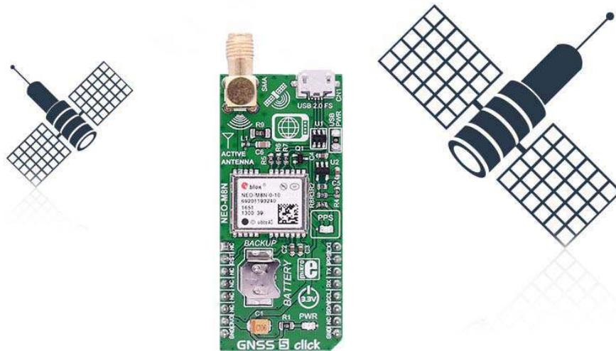
If the user wants to utilize GNSS to determine a position, they must have an antenna that receives the signals coming from the satellites, and a receiver that translates these signals. The antenna position will be deduced from the measurements of the time delay between the emission time (satellite) and the reception time (receiver) for at least 4 signals coming from different satellites.
