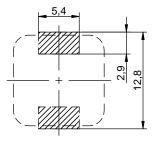
no sensitive traces underneath the component
