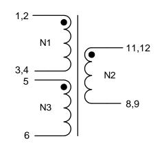
Application of the transformer allows for the leadwires between terminals 1&2, 3&4, 11&12, and 8&9 to solder bridge.
