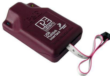
Figure 10-1: P&E's USB Multilink (USB-ML-12 shown)
