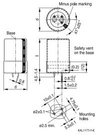
Snap-in terminals, length (6.3 + 1/-1.4) mm. Also available in a shorter version with a length of (4.5 - 1.4) mm. PET insulation cap is positioned under the insulation sleeve.
