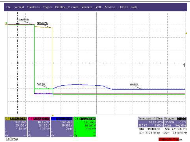
V_{IN A} = 54.5\text{ V} , V_{IN B} = 54\text{ V} , No Load, Scope GND = RTN
