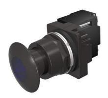
30mm BlackMax, Epoxy Coated Corrosion Resistant Complete Metal Unit Illuminated Push-Pull Operator Full Voltage, 12V AC/DC Incandescent Lamp Mushroom Head Cap Small 1 3/4" (44.5 mm) Metal, Black with Blue Lens 3 Position Pull-Momentary/Push-Maintained UL Listed, CSA Certified NEMA 1,3,3R,4,4X,12,13 & Automotive Standards
