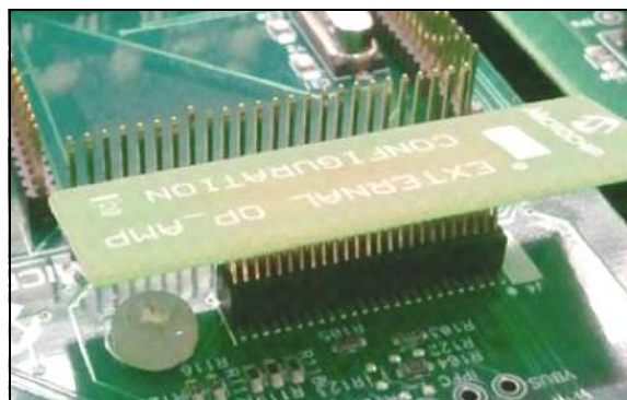
FIGURE 2: EXTERNAL OP AMP CONFIGURATION BOARD
