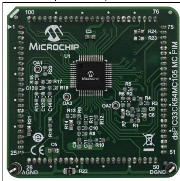
FIGURE 1: dsPIC33CK64MC105 EXTERNAL OP AMP MOTOR CONTROL PIM (MA330051-1)
