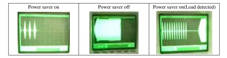
The Global LF Series is designed with extraordinarily low idle power consumption of 0.8-1.8% of its rated power.
