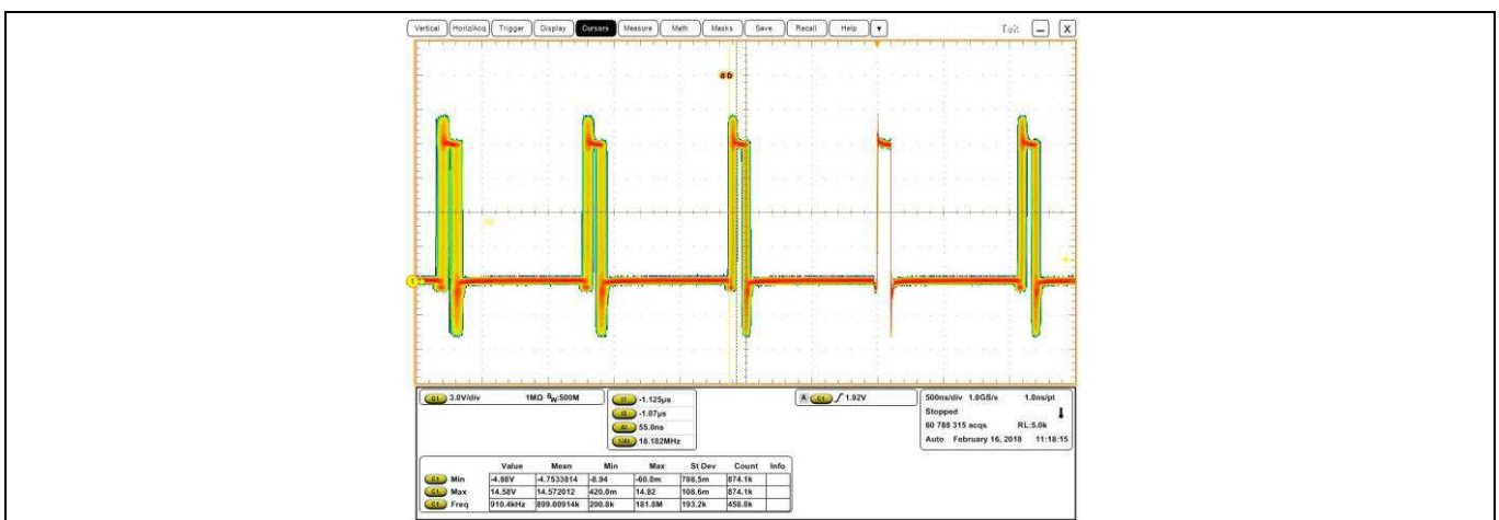
Figure 19 SW node, 25 A load, fsw = 800 kHz
