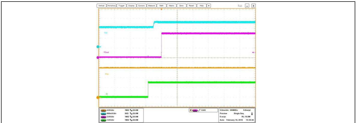
Figure 17 Pre-bias Start up at 0 A Load, (Ch1: PV in , Ch2: V out , Ch3:P Good ,Ch4:Enable)
