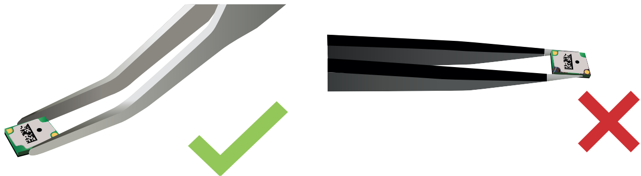
Figure 13: Left: Recommended tweezer type. Right: Not recommended tweezer type
