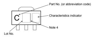
Note 4: A line under a Lot No. identifies the indication of product Labels. Not underlined: [[Pb]]/INCLUDES > MCV Underlined: [[G]]/RoHS COMPATIBLE or [[G]]/RoHS [[Pb]]
