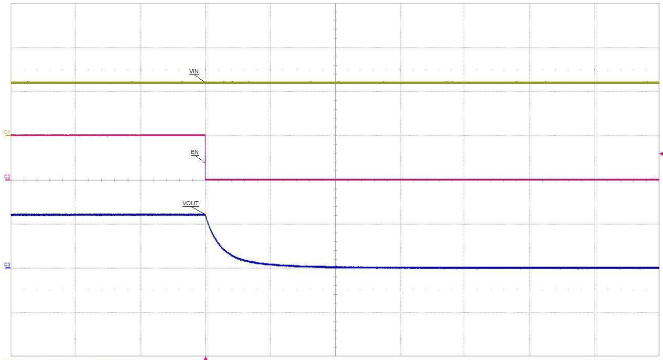
Figure 6. TPS22810 VOUT Fall Profile With QOD = VOUT (VIN = 12 V, CT = 22 nF, COUT = 10 \mu F, RL = 1000 \Omega )
