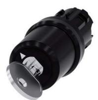
key-operated switch Siemens, 22 mm, round, plastic, lock no. LSG1, with 2 keys, 2 switch positions O-I, latching, actuating angle 90°, 10:30h/13:30h, key removal O+I, with laser labeling, upper case
