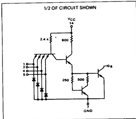
This device consists of two 4-input NAND gates with no output pull-up circuits. It can be used where the Wired-OR function is required or for driving discrete components.
