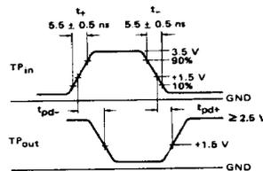
\*The coax delays from input to scope and output to scope must be matched. The scope must be terminated in 50 ohm impedance. The 950 ohm resistor and the scope termination impedance constitute a 20:1 attenuator probe. Coax shall be CT-070-50 or equivalent.
