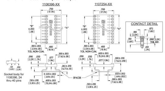
**ALL DIMENSIONS: INCHES [MILLIMETERS]** ALL TOLERANCES: ±0.005 [0.13] UNLESS OTHERWISE SPECIFIED CONSULT FACTORY FOR OTHER SIZES AND CONFIGURATIONS
