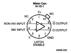
Note: On metal package, pin 5 is connected to case. On DIP, pin 6 is connected to case.
