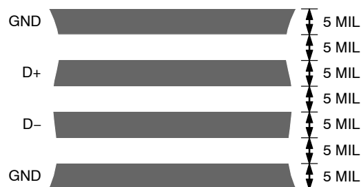
Figure 28. Arrangement of Signal Tracks
