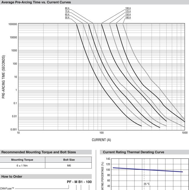
DERATING PERCENTAGE (%) POWrFuse™ 20 Product Designator Series Name 0 -40 -60 -20 0 20 Mounting Type -B1 = Bolt Mounting, Type 1 AMBIENT TEMPERATURE (°C) Rated Current 50 - 180 = 50 A - 180 A
