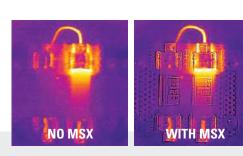
PRODUCE CRISP THERMAL IMAGES See the detail needed to troubleshoot faults and gauge their severity
