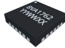
24-lead 4mm x 4mm x 0.9mm QFN
