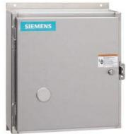
Mechanically held lighting contactor, Contactor amp rating 30Amp 0NC  $\_$  5NO poles, 277VAC 60HZ coil, Non-combination type, Encl NEMA type 4X 304 S-steel Water/dust tight noncorrosive
