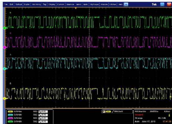
THVD2450 V_{CC} = 5\text{ V} R_L = 50\ \Omega Random (PRBS7) data at 50 Mbps
