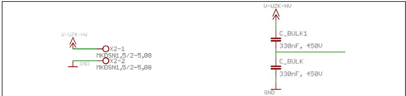
Figure 13 HV supply input (left) and DC-Link connection (right)
