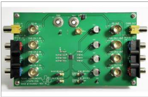
THS7372PWEVM, the THS7372 Evaluation Module, Top View
