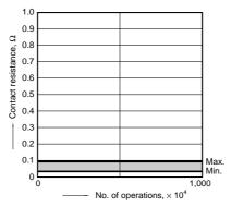
2-(2). Change in dynamic contact resistance (10 μA 1 mV DC resistive load) Tested sample: ASX20012, 10 pcs.
