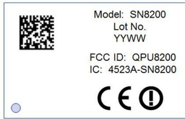
FIGURE 7.2 Typical SN820X/820XUFL module marking
