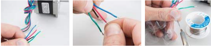
Left: the wire ends look pretty ratty from the factory. Center: Collect the wire strands by giving them about 180 degrees of twist along the length of the strip. Right: Tin each lead. Apply excess solder to allow the flux to work, and pull the extra solder off with the iron yielding a solid cylinder of wire.
