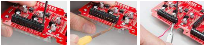
Left: Back the screw out until flush. Center: Gently open the contact plate. Right: Help put the wire in with a tool that is choked up near the tinned end. You can't push a rope!
