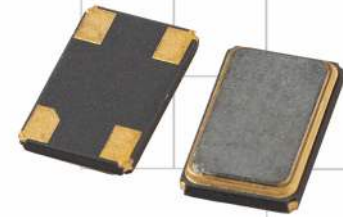
Part Dimensions: 5.0 × 3.2 × 1.65mm • 60.7734mg
