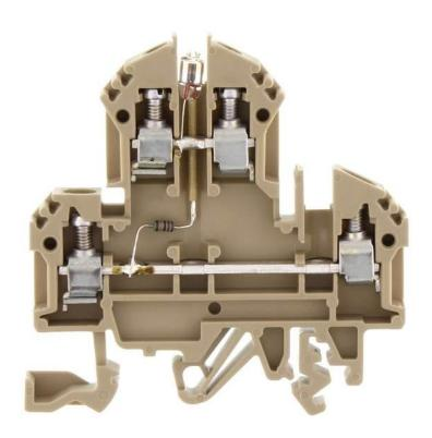
Double-level terminal with electronic components, Screw connection, Mounting type:Mounting rail TS 35/7.5 and TS 32, Rated cross-section: 4 mm², Width: 6 mm, Colour: Beige
