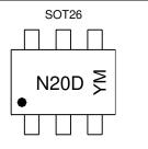
N20D = Product Type Marking Code YM = Date Code Marking Y or  $\overline{Y}$  = Year (ex: C = 2015) M or  $\overline{M}$  = Month (ex: 9 = September)
