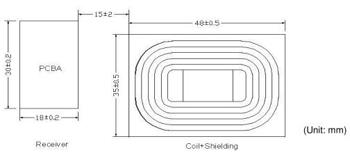
PCBA : 30 \* 18 \* 1.6 mm (Max.) Coil + Shielding : 48 \* 35 \* 1.5 mm (Max.) Amount of space between the PCBA to Coil+Shielding as follows: 15 ± 2 mm
