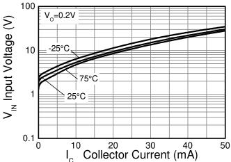
Input Voltage v Collector Current
