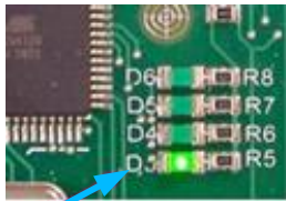
Figure 5. D3 Status LED for MCB Microcontroller
