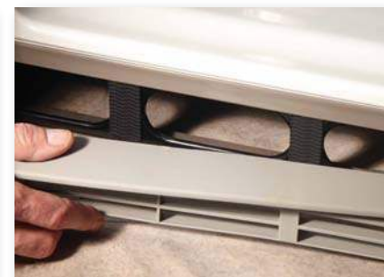
Hold plastic air vent to base of refrigerator with strength to resist vibration
