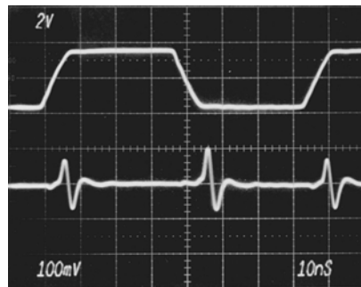
Switching Glitch, 0V to 0V with 10ns AB Edges
