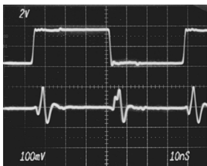
Switching Glitch, 0V to 0V with 2ns AB edges
