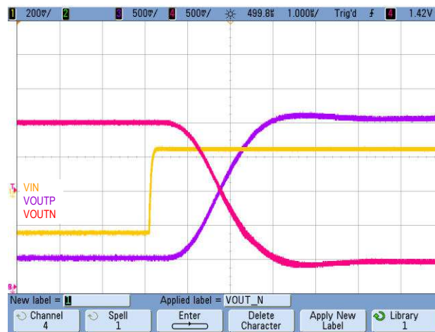
Figure 8-4. Step Response of the AMC1301-Q1
