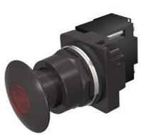
30mm BlackMax, Epoxy Coated Corrosion Resistant Complete Metal Unit Illuminated Push-Pull Operator Transformer type, 600V AC LED Lamp Mushroom Head Cap Small 1 3/4" (44.5 mm) Metal, Black with Red Lens 3 Position Pull-Momentary/Push-Maintained UL Listed, CSA Certified NEMA 1,3,3R,4,4X,12,13 & Automotive Standards
